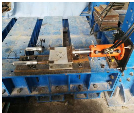
Fig. 3. Dampers performance test.
