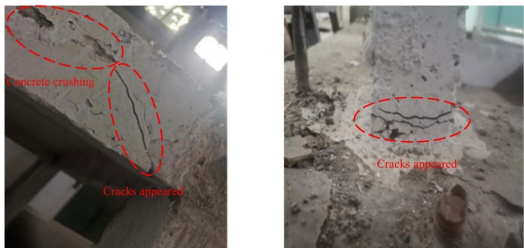
Fig. 6. Failure phenomenon of 0.8 g peak acceleration.
