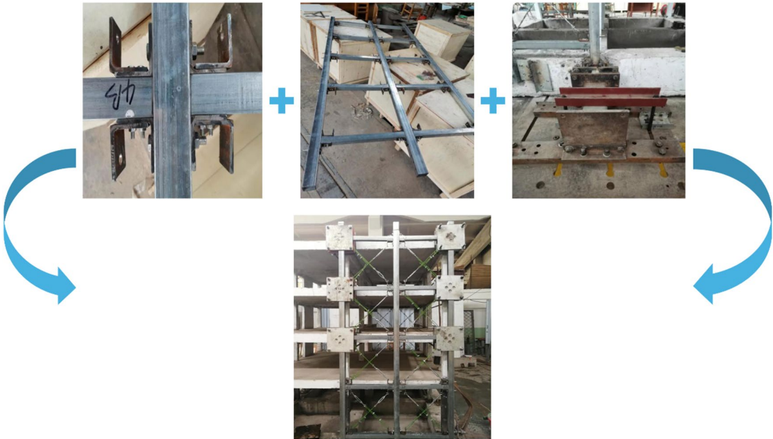
Fig. 1. Fabrication and installation of external steel frame.
