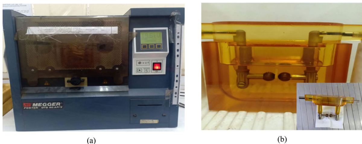
Fig. 4. (a) Megger Foster 60AF/2 Oil tester, (b) Test step.
