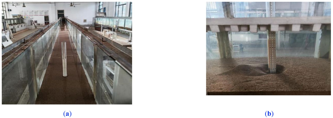
Fig. 4. Experimental Site Photograph: (a) flume; (b) pier scour.
