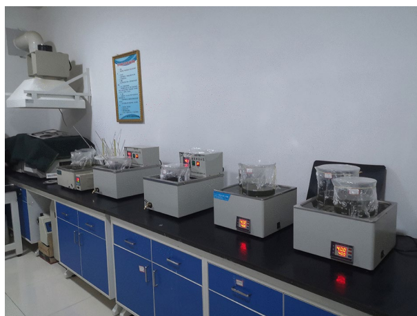
Fig. 4. Scene of water bath heating in same-year brine mixing laboratory experiment.
