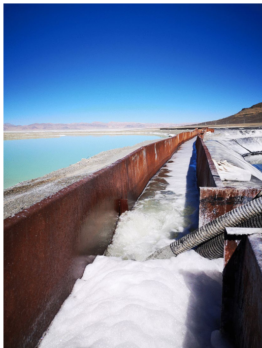
Fig. 9. Scene of brine mixing in brine delivery channel in cross-year brine mixing production test.
