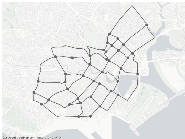
Fig. 1. Routing Network in Singapore. The nodes represent aerodromes, while the lines represent corridors. This airspace structure was generated using the OneSky UTM simulator.
