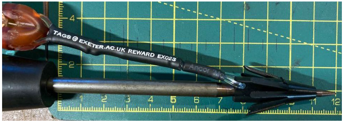
Fig. 2. An example of the metal tag applicator used to deploy pop-up satellite tags (PSAT) on BFT. Swabs of the applicator and the stopper bung were taken after tagging to sample the DNA of the tagged individual.
