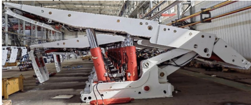
(b) Canopy in a "high angle" position ( l_1 = 2550\text{mm}, l_2 = 2285\text{mm}, l_{19} = 956\text{mm} )
