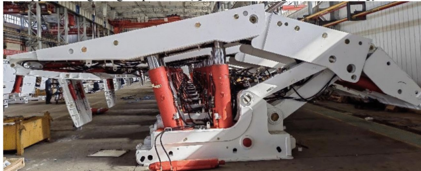
(c) Canopy in a "downtilt" position ( l_1 = 2100\text{mm}, l_2 = 2298\text{mm}, l_{19} = 1001\text{mm} )
