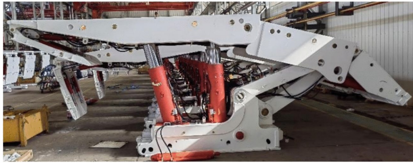
(a) Canopy is essentially parallel to the base ( l_1 = 2305\text{mm}, l_2 = 2335\text{mm}, l_{19} = 1009\text{mm} )
