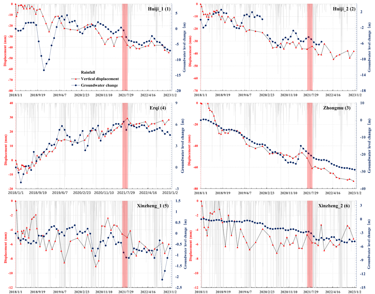
Fig. 7. Time series of vertical displacement derived by StaMPS-SBAS method and groundwater level changes at six wells during the period January 2018 and December 2022 in Zhengzhou city: (1) Huiji_1, (2) Huiji_2, (3) Zhongmu, (4) Erqi, (5) Xinzhen_1, and (6) Xinzhen_2 corresponding to the location (1)–(6) in Fig. 1. The grey bar indicates the daily rainfall schematic diagram, whose length corresponds to the daily precipitation, with a longer bar indicating heavier rain on that day. The red vertical bar represents the moment of the extreme rainstorm event in July 2021. All groundwater level changes in the graph are observed in well data.
