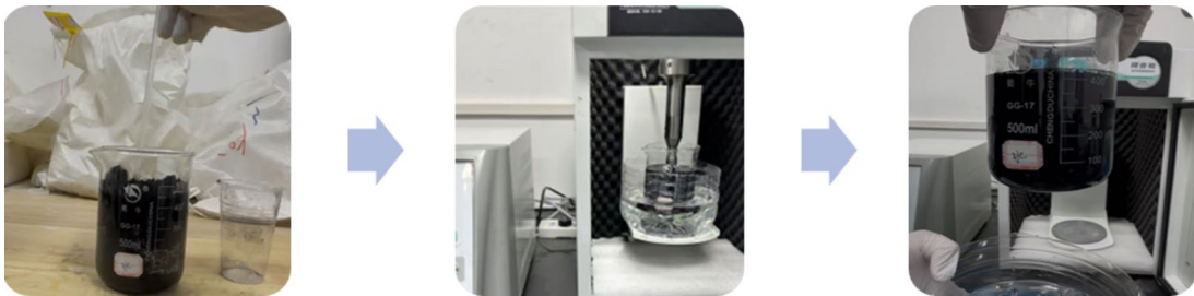
Fig. 4. The dispersion process of MWCNTs.
