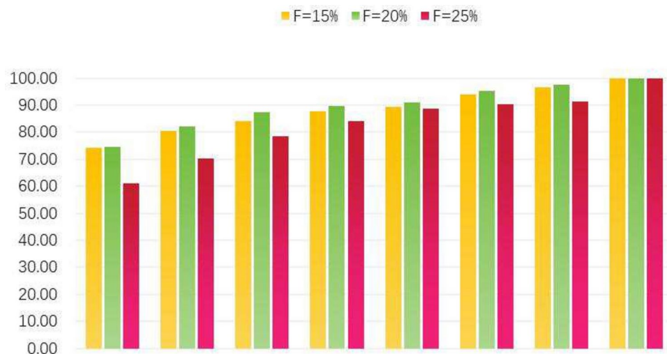
Fig. 7. Relationship between Concrete Elastic Modulus and Fly Ash Content.
