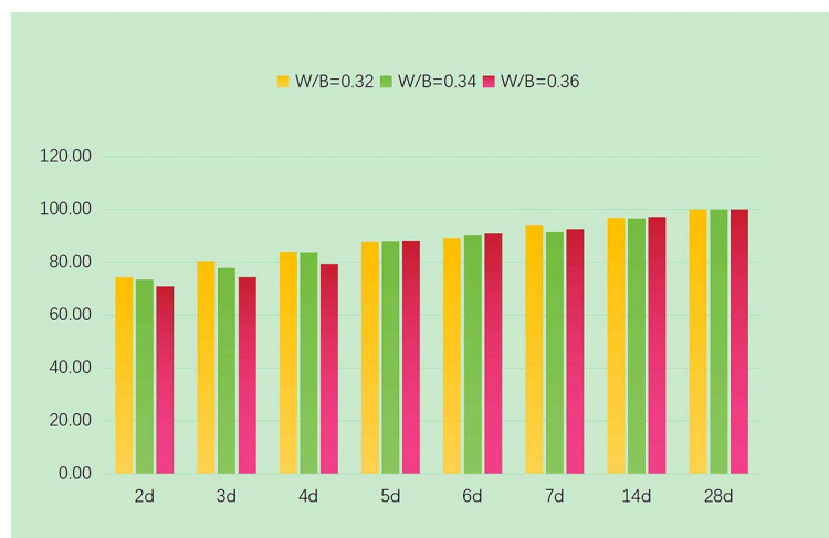
Fig. 8. Relationship Between Concrete Elastic Modulus and Water-Cement Ratio.
