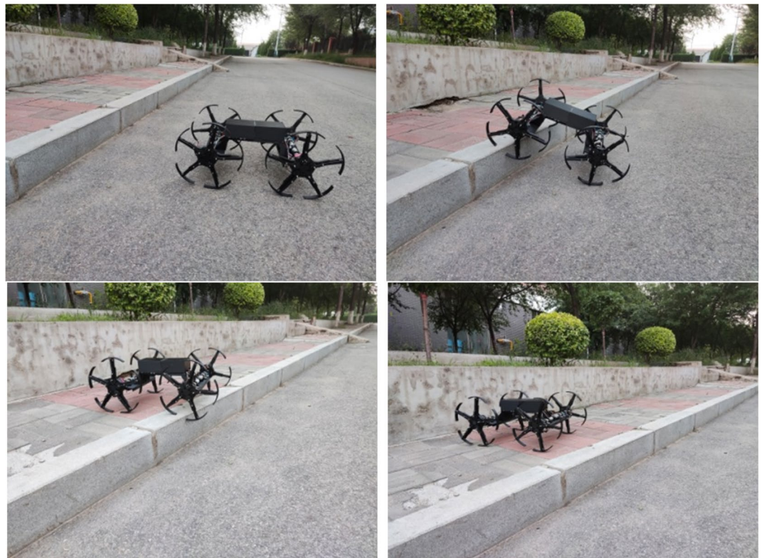
Fig. 16. Obstacle surmounting process of robot.
