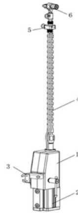
1.Main Unit 2.Cylinder 3.Surgical Bed Clamp 4.Flexible Robotic Arm 5.Pneumatic Button 6.Instrument Holder
