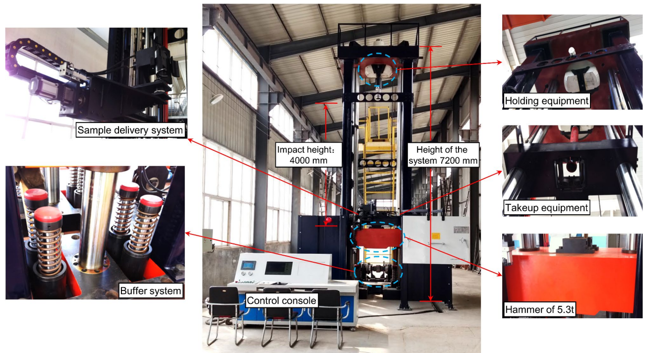
Fig. 1. Dynamic pull-out test system with drop hammer.
