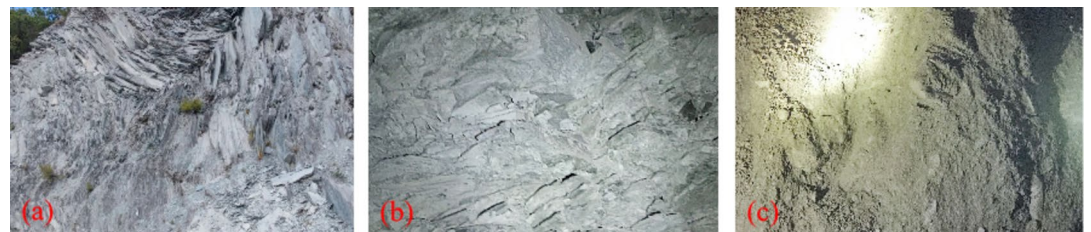
Fig. 2. Foliated metamorphic basalt. (a) Observed in surface outcrops; (b) Exposed foliated metamorphic basalt during tunnel excavation; (c) Weathered schistosized basalt after several hours.
