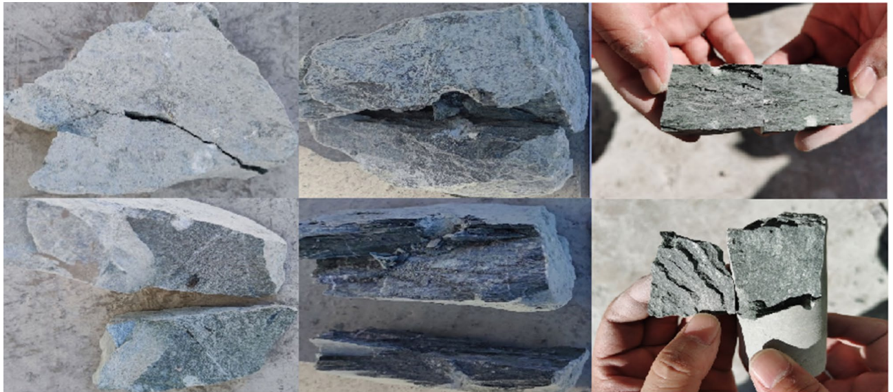
Fig. 11. Failure modes observed in PLT for foliated metamorphic basalt.
