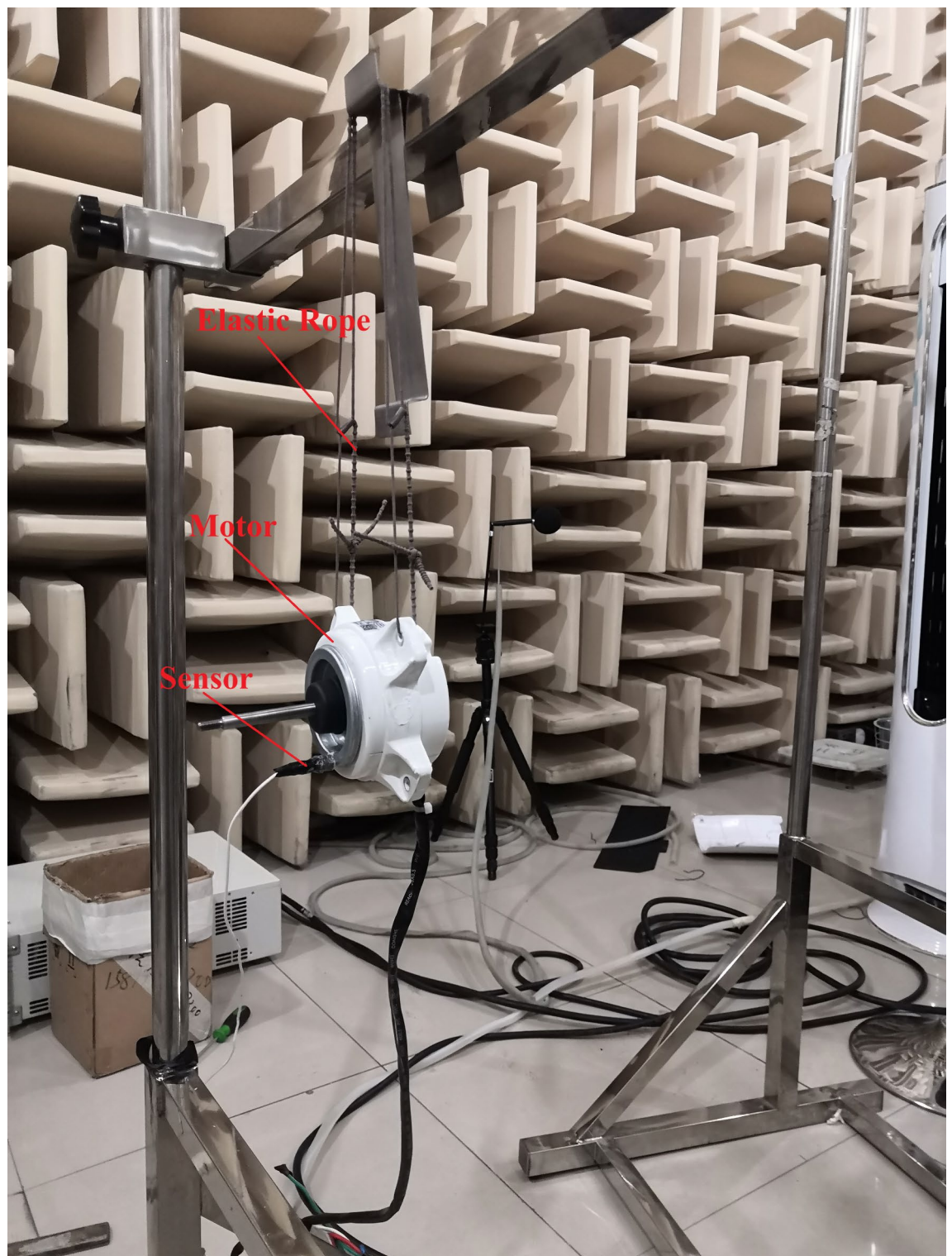
Fig. 7. Vibration test chart of single motor.
