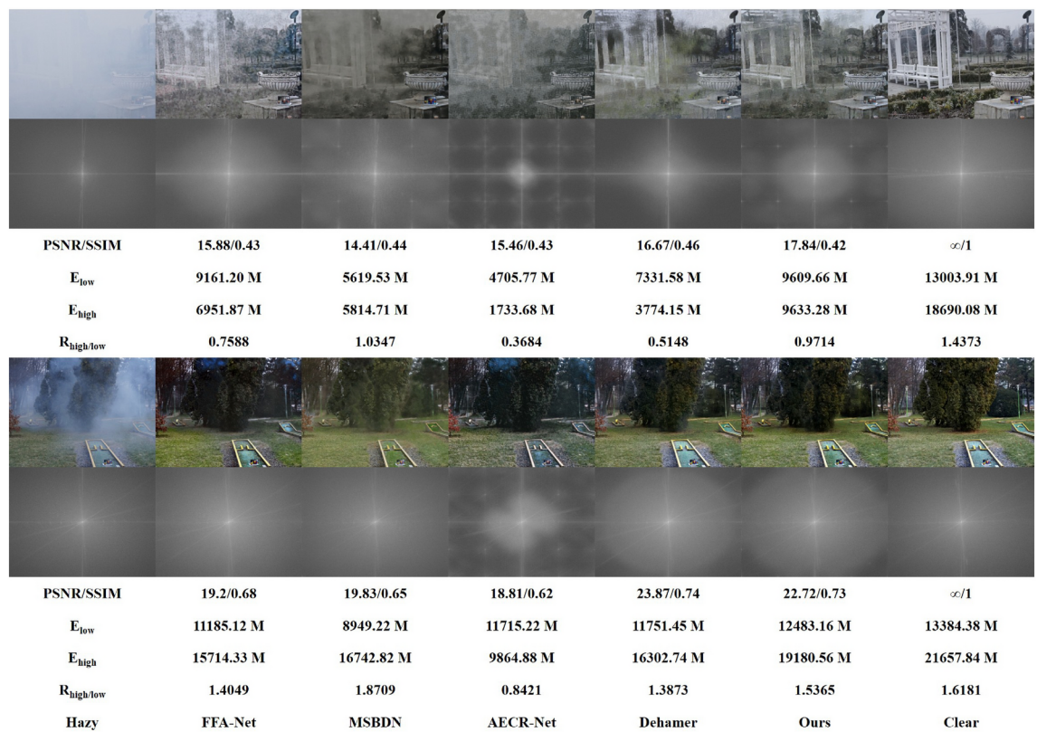
Fig. 4. Visual and frequency domain comparison of different dehazing methods on Dense-Haze and NH-Haze datasets. The images above are from Dense-Haze and their corresponding spectral plots. The images below are from NH-Haze and their corresponding spectral plots. PSNR and SSIM refer to the values obtained by comparing the images above with the original images. E_{low} and E_{high} represent the low and high-frequency energy of the spectral plots above, respectively. The closer these two values are to the low and high-frequency energy of the clear image, the better. R_{high/low} , when the low and high-frequency energy is close to that of the clear image, should be as close to the clear image as possible.
