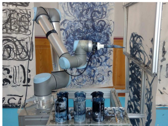
Fig. 1. Physical setup comprising the magnetic painting frame and the 6-DOF robotic arm (UR10) with attached FT sensor and brush holder. Impression of the room installation Synaesthetic Strokes (2023) at the Collegium Helveticum. Photo by Marcus Nebe, ©VG Bild Kunst / Liat Grayver.
