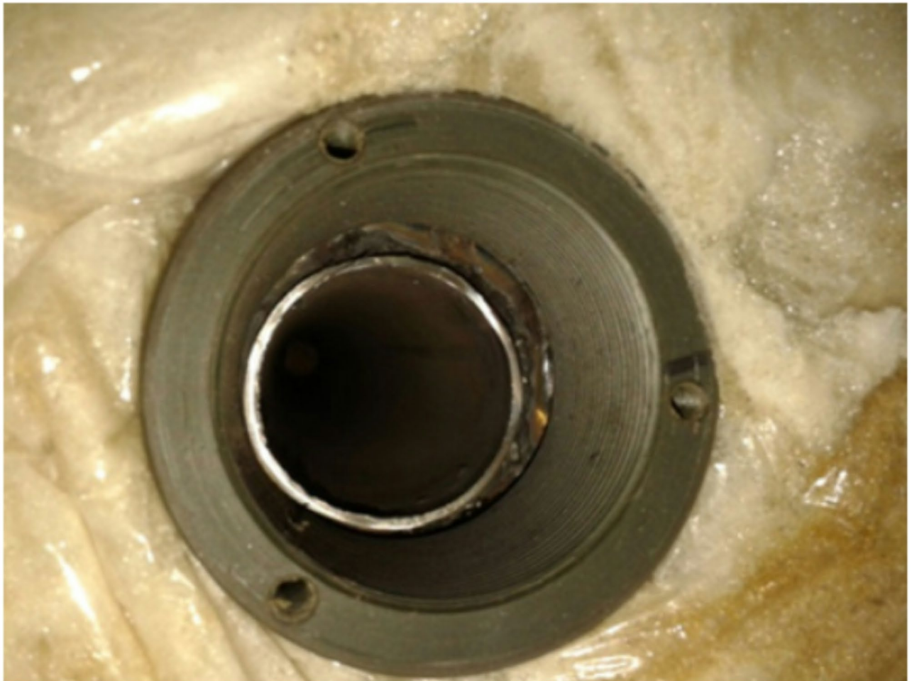
Fig. 3. Placement of heater for HTF in each heat exchanger.
