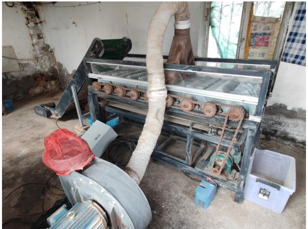
Fig. 11. Airflow-disc sieve type film separation test bench.
