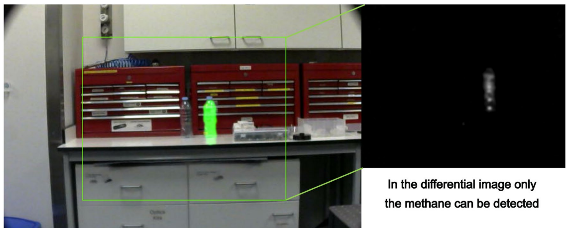
Fig. 3. Image taken using the gas imaging device of two clear bottles, one containing butane and the other containing methane. It can clearly be observed that only the methane bottle returns the bright green gas signature, highlighting the specificity of the absorption band selected for investigation. This is further highlighted in the insert which shows the processed differential SWIR image, where signal is only present for in the region of methane gas.
