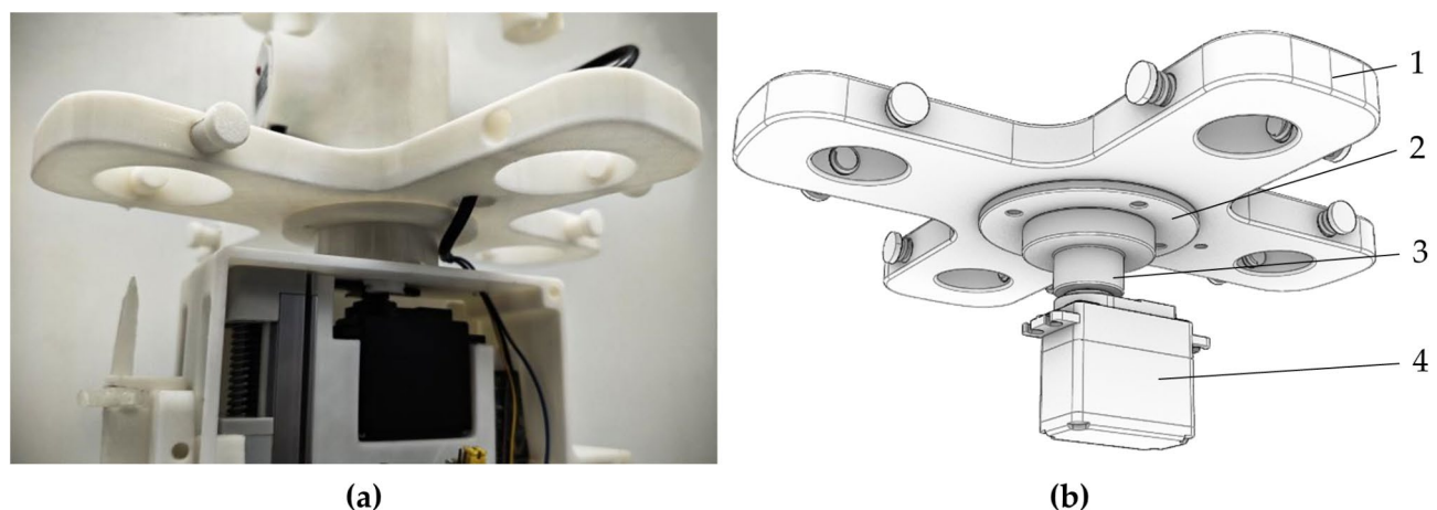
Fig. 8. Schematic of the rotational medication replacement mechanism: (a) actual photograph of the mechanism and (b) model diagram of the mechanism (1. lower securing platform, 2. connecting disc, 3. flange, 4. servo motor).
