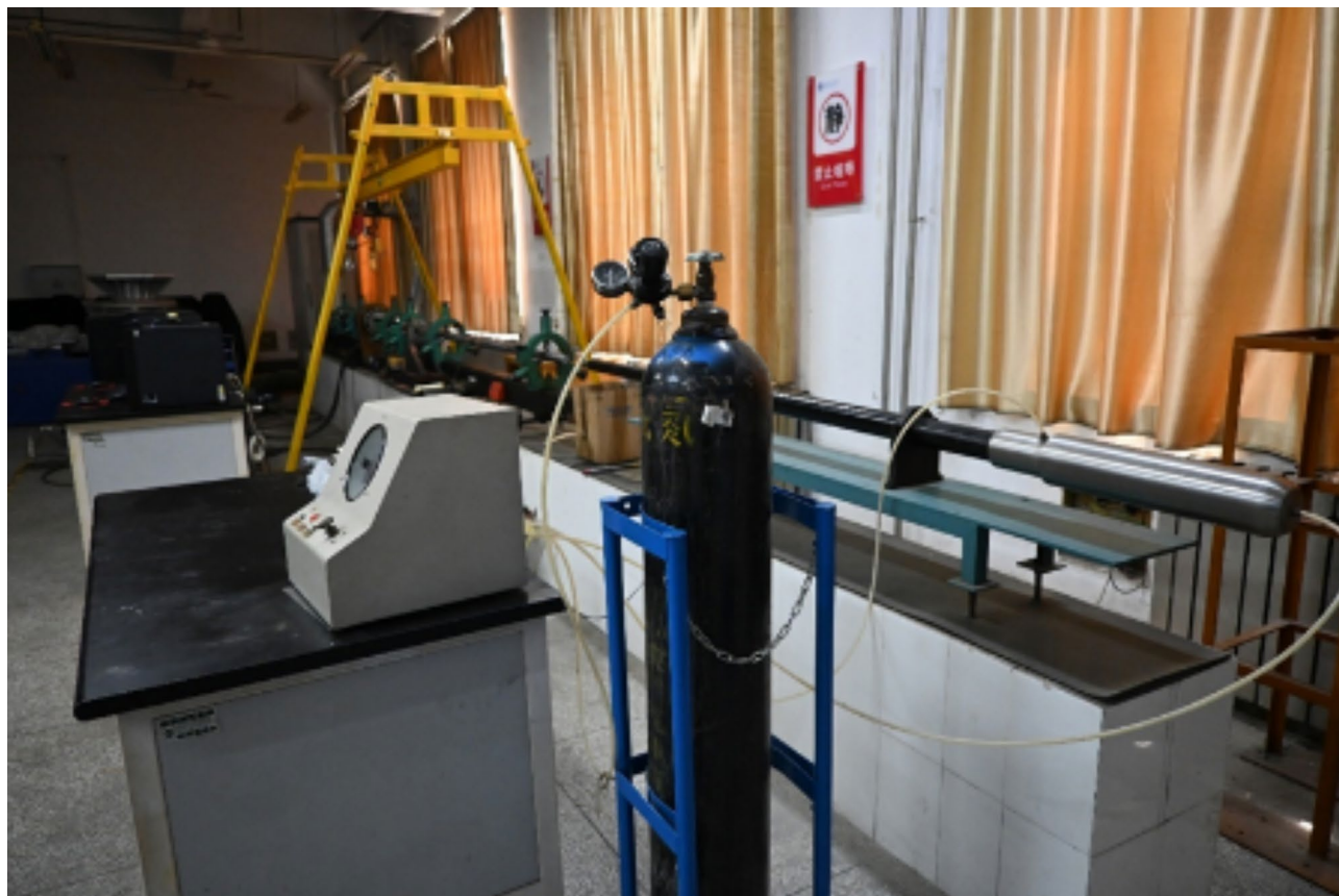
Fig. 3. Diagram of pneumatic split Hopkinson lever device.
