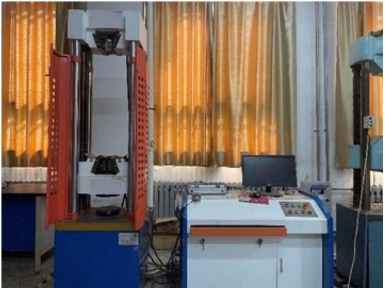
Fig. 2. Electro-hydraulic servo universal testing machine.
