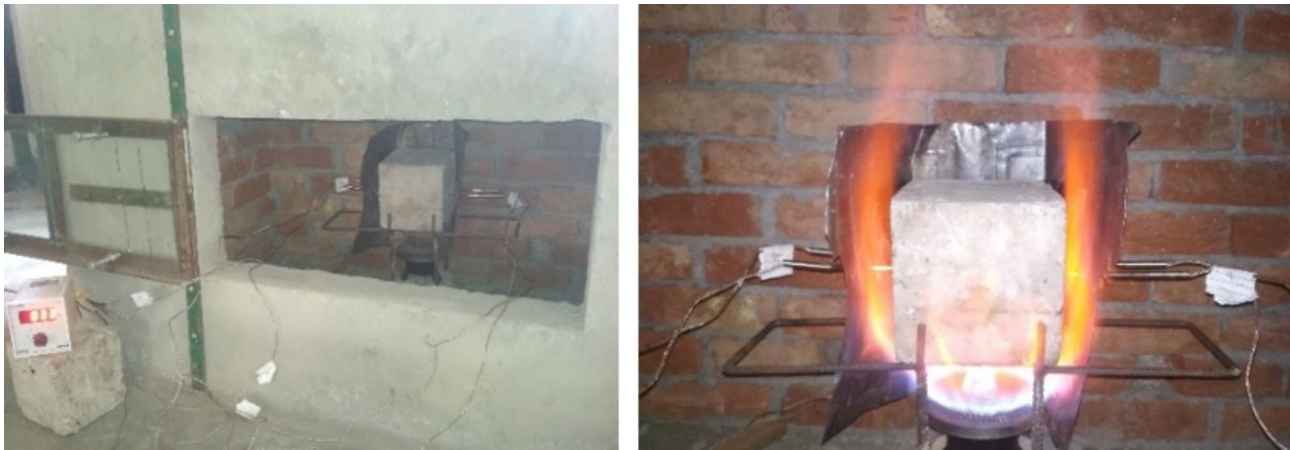
Fig. 2. Photographs of open fire testing for the CBC samples.
