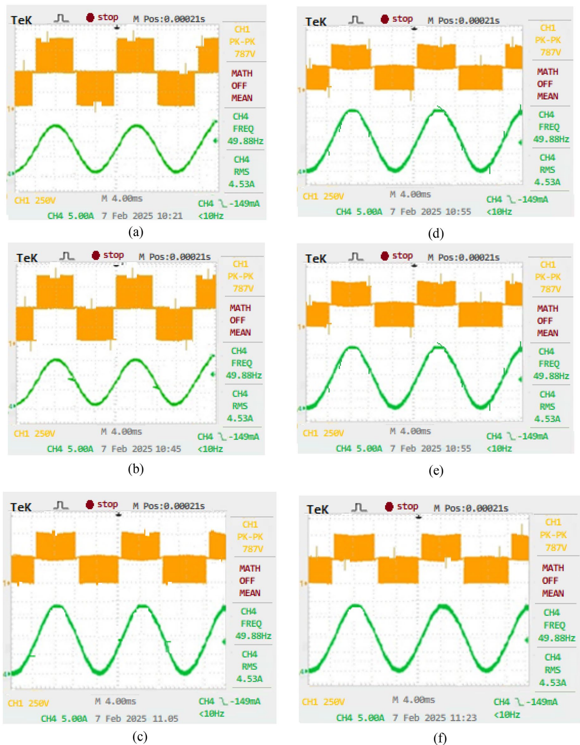
Fig. 10. Experimental test results of differential mode output voltage ( V_{AB} ) and output load current ( i_{out} ) for (a) Heric, (b) HBZVR, (c) HBZVSCR, (d) PN-NPC, (e) H6-I and (f) proposed H6-D TL-PVI topologies.
