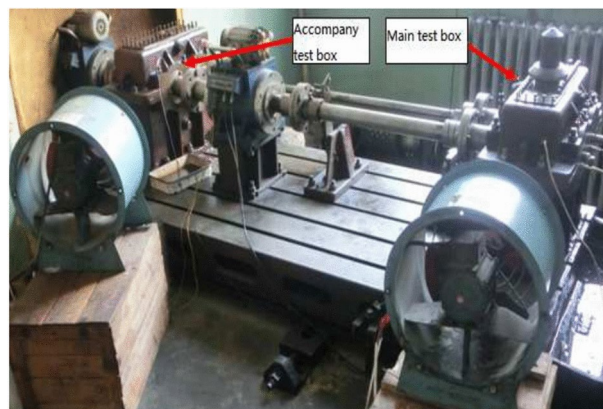
Fig. 3. Gear fatigue test bench.
