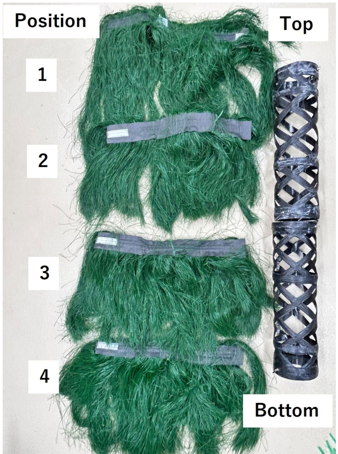
Fig. 3. The plastic sheets were wrapped around cylinders (1 m long, 14 cm diameter) to make the artificial seaweed. Each artificial seaweed was wrapped by four plastic sheets. The seaweed units were numbered from 1 to 4, starting from the top of the cylinder to enable the estimation of the number of eggs deposited in each region of the seaweed.
