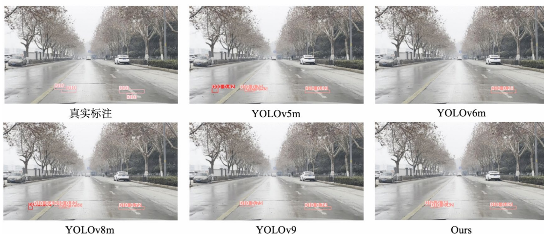
Fig. 18. Visualization of detection results of different detection models for a single category of damage in a complex environment.
