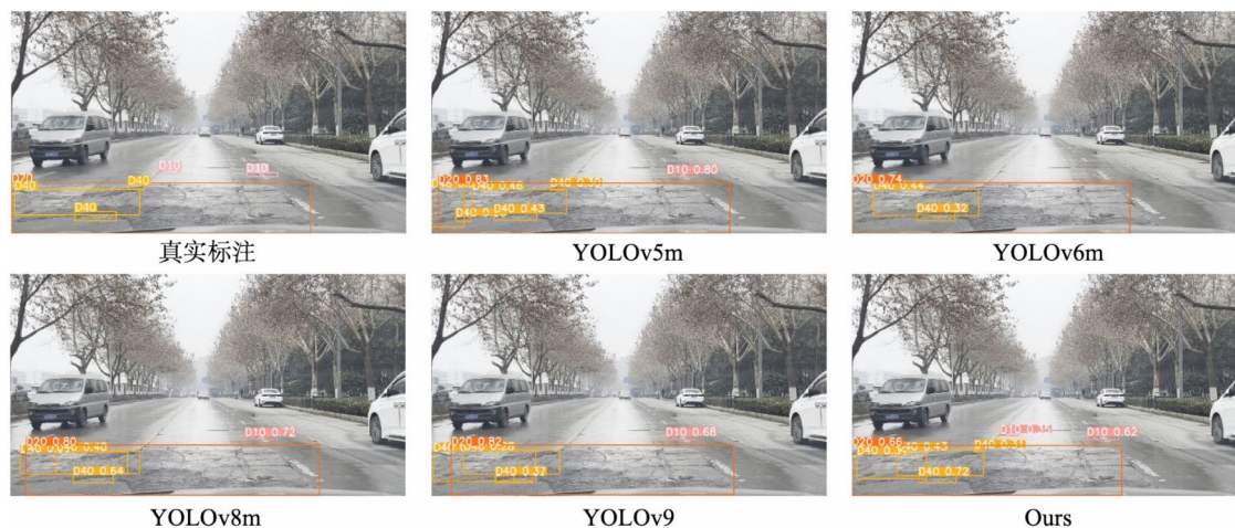
Fig. 20. Visualization of detection results of different detection models for multiple categories of damage in a more complex environment.
