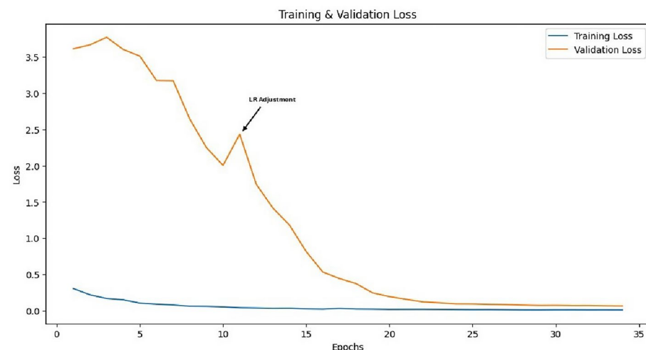
Fig. 3. Training and validation loss while training 1D CNN model on SAVEE dataset.
