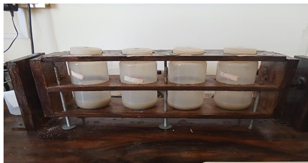
Fig. 10. Experimental setup for leachability test.
