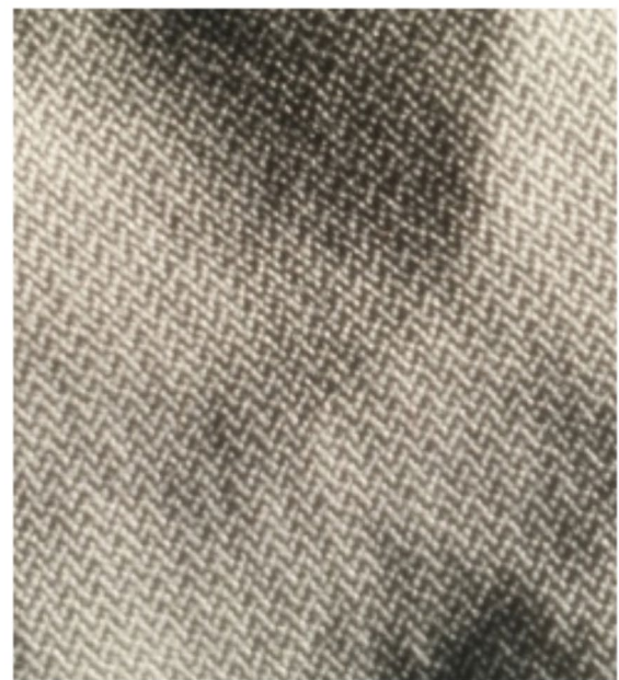
PAD 6.6 woven (fiber mean surface roughness 0,082 \mu\text{m} )
