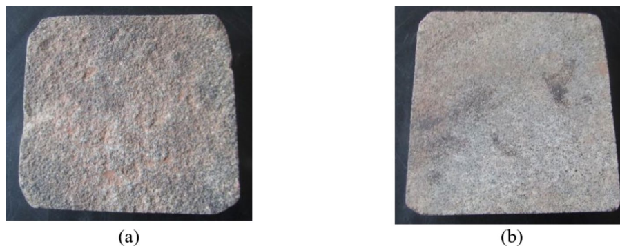
Fig. 16. Bedrock for the shear test. (a) Rough bedrock; (b) smooth bedrock.
