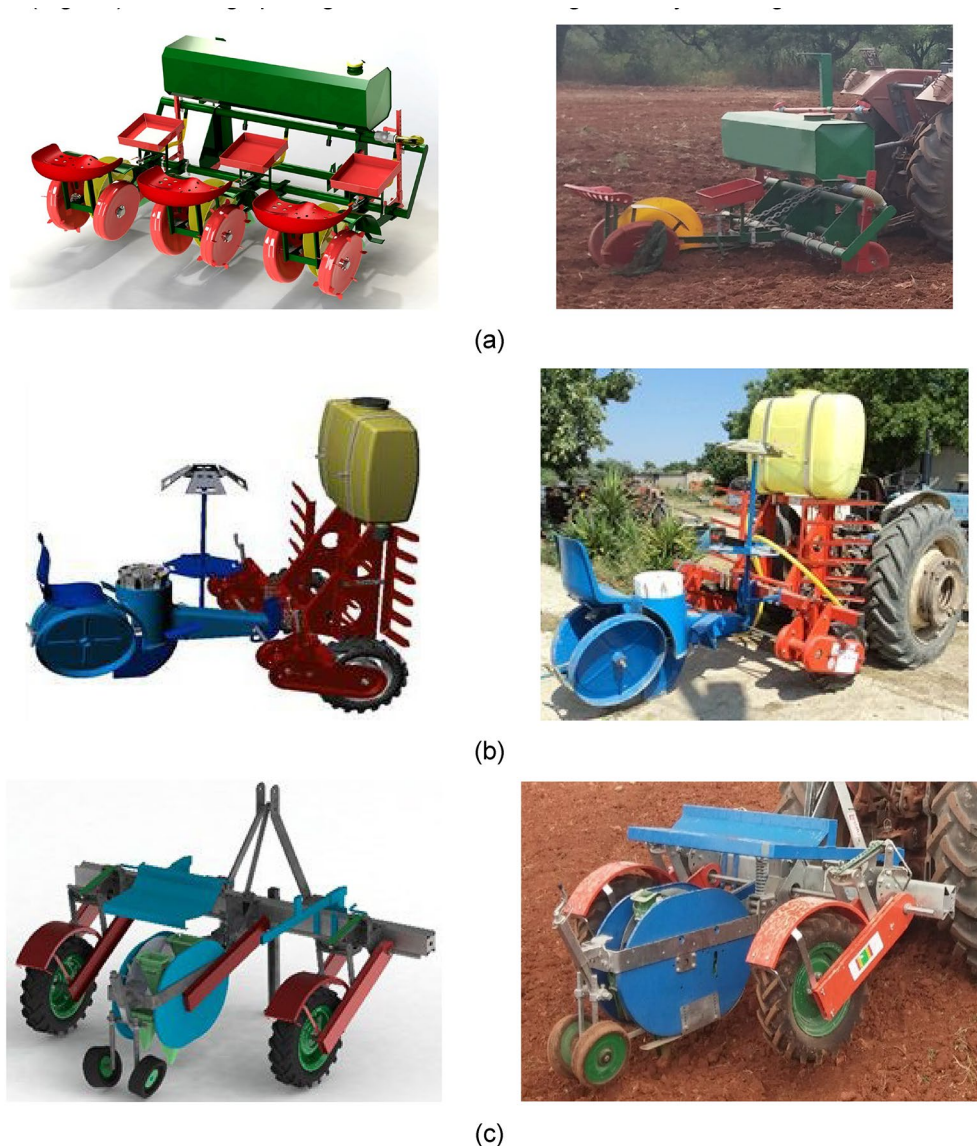
Fig. 2. Transplanters evaluated in this study for potted seedling transplantation under different tillage conditions: (a) disc-type transplanter with elastic discs to minimize seedling damage and markings for spacing adjustment, (b) carousel-type transplanter with automated seedling placement and press wheels for compression, and (c) dibble-type transplanter with a funnel mechanism for precise seedling deposition.
