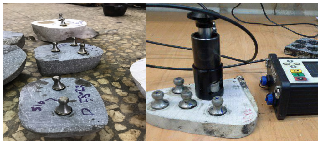
Fig. 4. Preparation and placement of samples in the Pull Off test.
