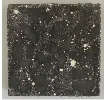
Fig. 2 Concrete pore structure test specimen
