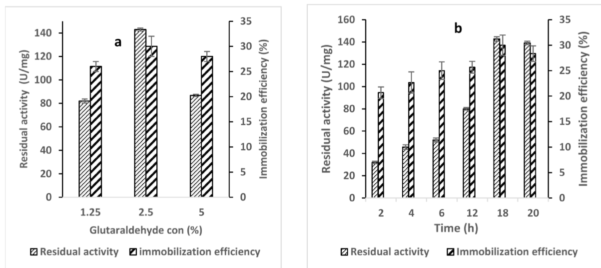
Fig. 2. (a) Optimization of glutaraldehyde concentrations and (b) time of coupling for LDP immobilization on the support.
