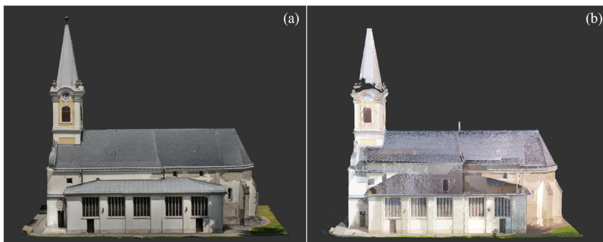
Fig. 4. Aerial-based Data Sets: (a) Drone Photogrammetry Data Set (b) TLS 2 Data Set. Image credit: photograph by R. Salah, CC BY 4.0.
