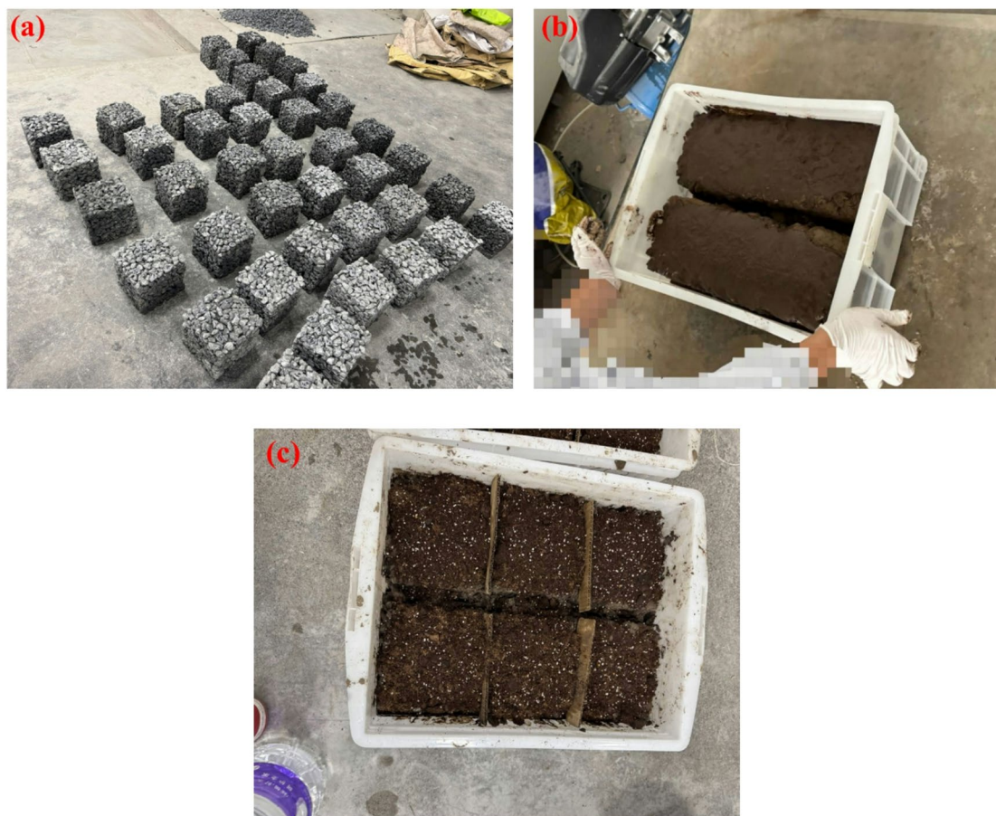
Fig. 2. On-site seeding of ecological concrete specimens after 28 days of curing.
