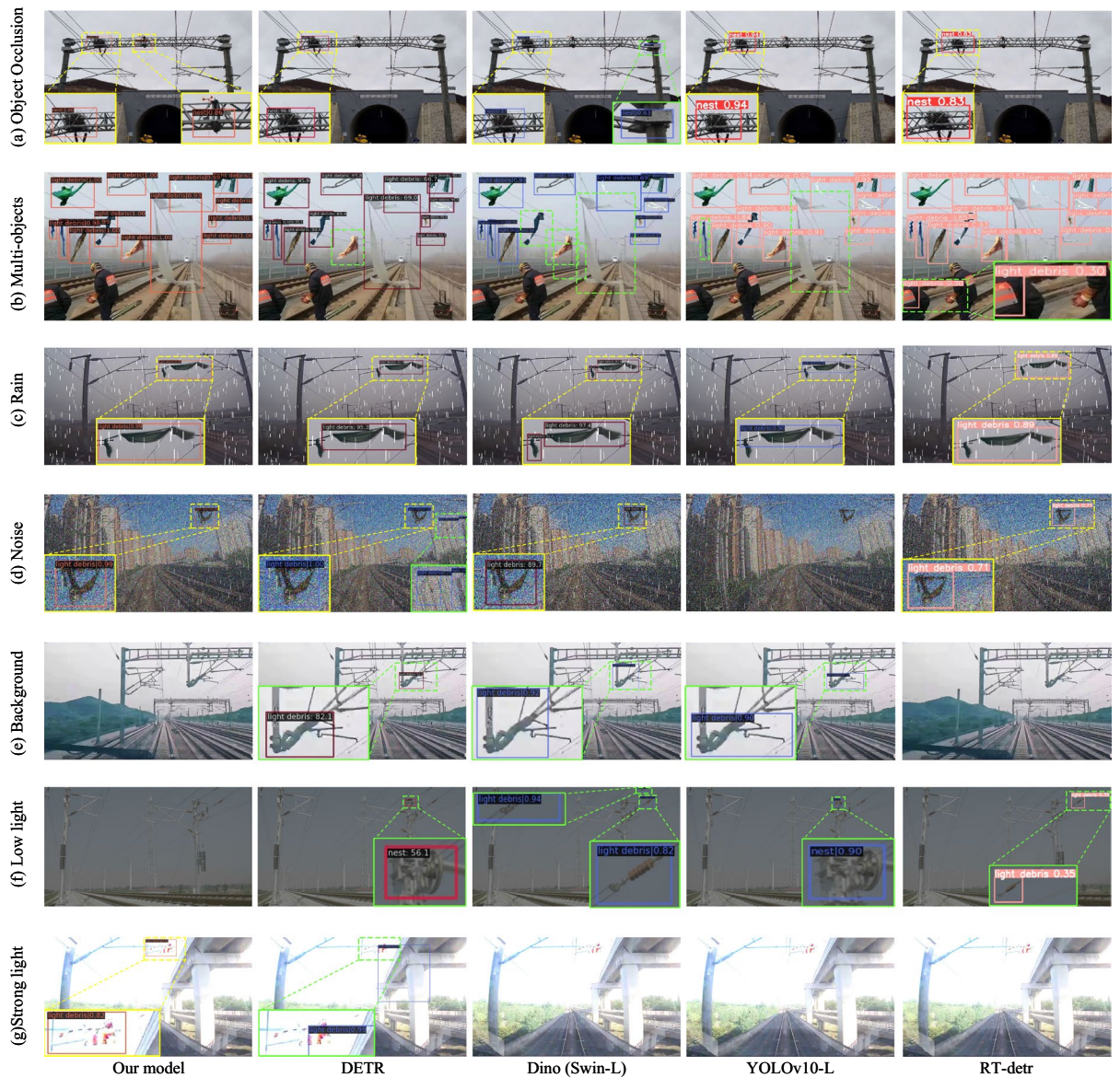
Figure 9. Comparison of the visualization of detection results between this method and other mainstream object detection methods on the RailCatFOD-DS Dataset.
