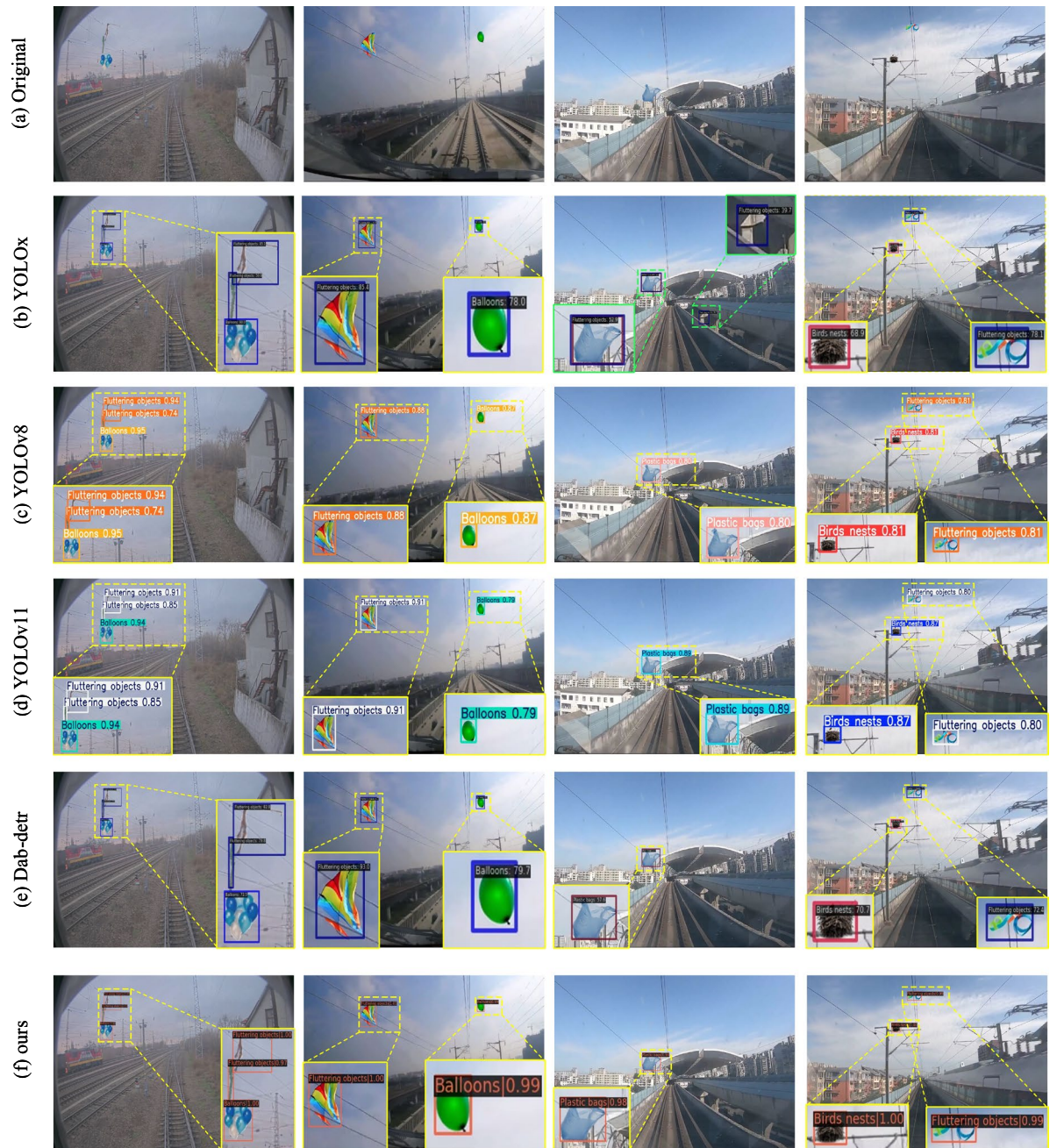
Figure 13. Comparison of the visualization of detection results between this method and other mainstream object detection methods on the RailFOD23 dataset.
