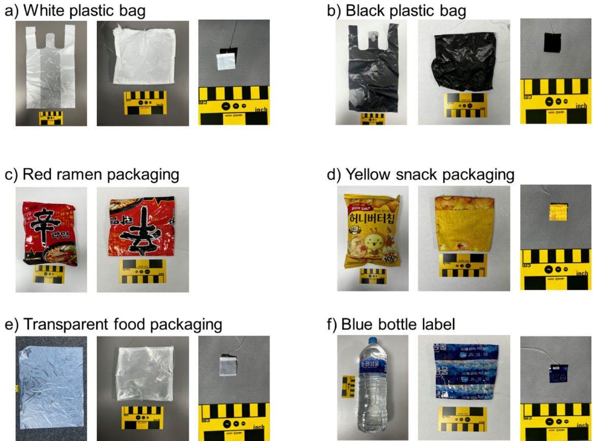
Fig. 1. Images of intact plastic film products and plastic stimuli used in the experiments for juvenile and post-hatchling turtles. For each plastic type, the leftmost item is the original product, the middle item was used as a stimulus for juveniles, and the rightmost item was used as a stimulus for post-hatchlings. Each small yellow and black bar on the scale indicates 1 cm, and the large bar indicates 1 inch.
