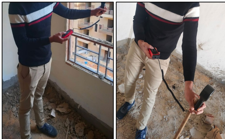
Fig. 4. Air speed measurements inside the building.
