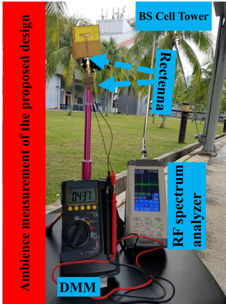
Fig. 10. Measurement setup for RFEH validation of the proposed antenna.
