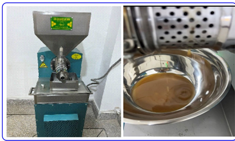
Fig. 3. Oil press of Opuntia Ficus indica seeds of Eastern Morocco.
