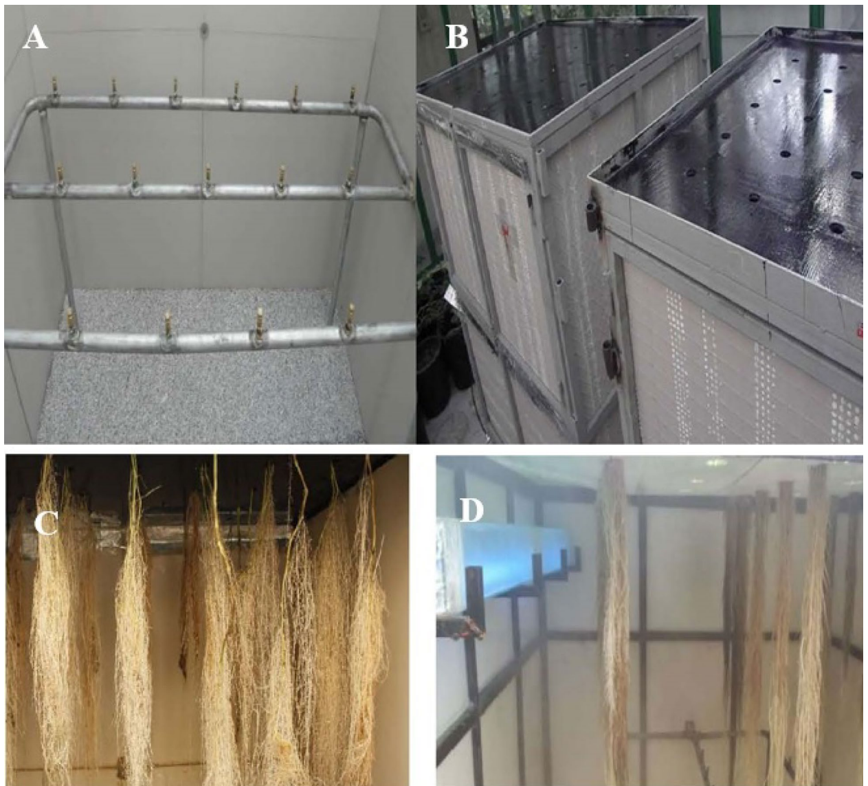
Fig. 1. Schematic and operational view of the phytorhizotron system. (A) Overhead section showing shoot development under controlled photoperiod. (B) Sealed down-Sect. (180 cm depth) where roots are exposed to 24-h UV-B radiation via side-by-side Philips TL40W/12/RS lamps.
