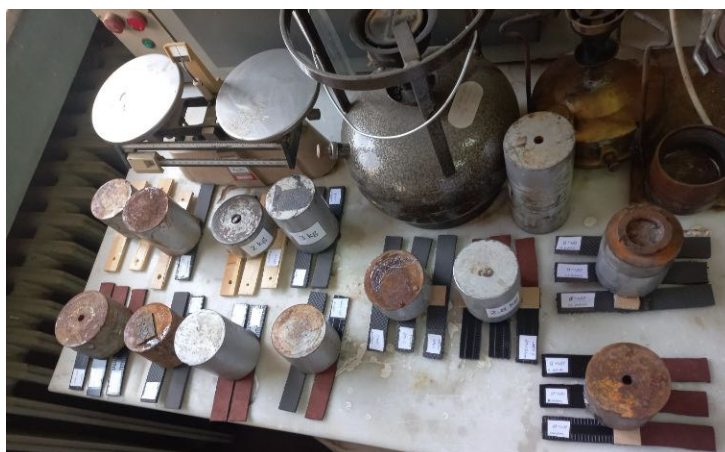
Figure 3. Labeled experimental samples prepared for tensile adhesion testing.
