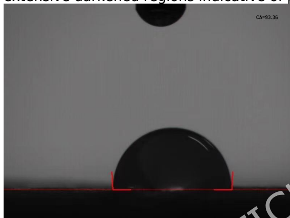
Figure 5. Contact angle images of moulded LDPE material.
