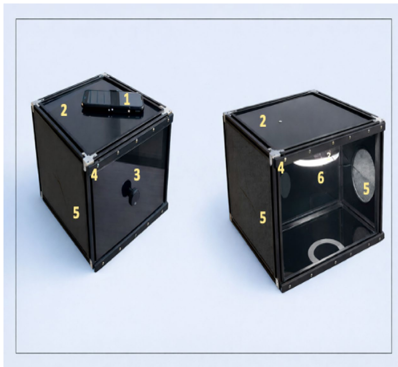
Fig. 9. Schematic representation of the SKINREMS device showing the conceptual design of the measurement chamber, illumination system, camera positioning, and subject stabilization developed by an interdisciplinary research team. 1 - Camera, 2 - Plexiglass plate, 3 - Sliding wall handle, 4 - Aluminum profile, 5 -Foam cut-out wall for forearm placement, 6 - Ring lamp.
