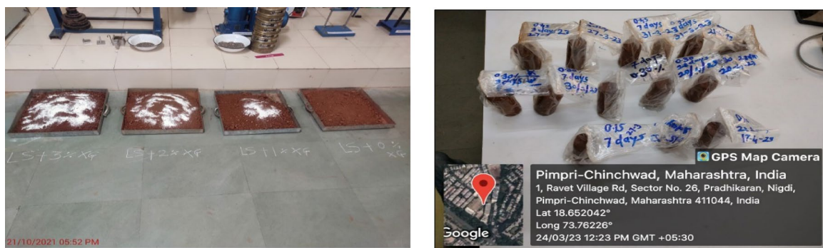
Fig. 7. (a) LS + XG (Dry Mixing) (b) Airtight UCS specimens.
