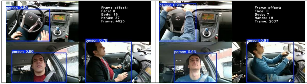
Figure 8. Visualized Detection Results of YOLOv11n* for Driver Monitoring.
