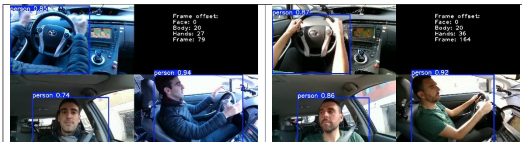
Figure 7. Visual Detection Results of YOLOv11n for Driver Monitoring.
