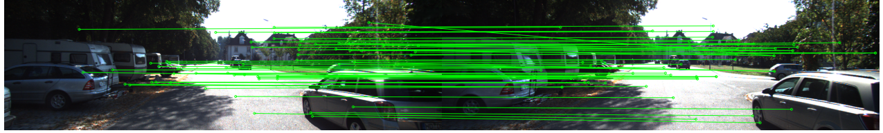
(b) Feature matching with class-wise semantic constraints, where cross-class mismatches are suppressed.
