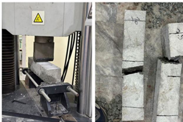
Fig. 11. Photographs of flexural strength test setup and failure patterns of beam specimens, showing crack propagation and fracture surfaces for control and ceramic waste concrete mixtures.
