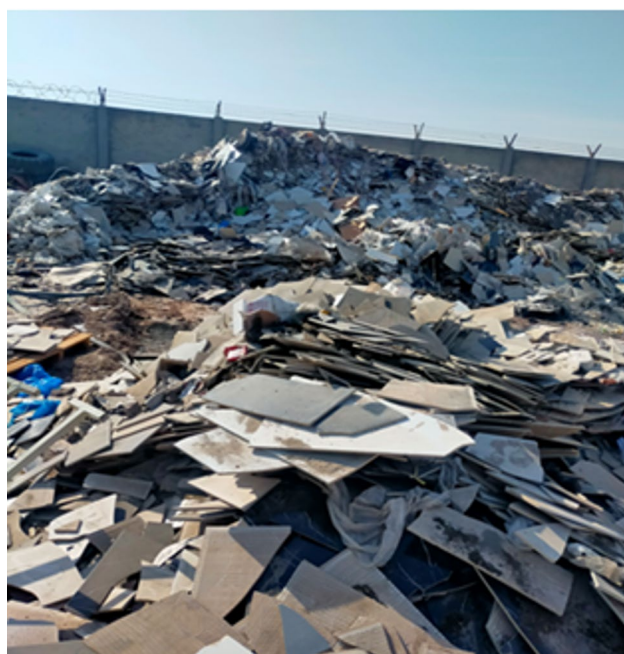
Fig. 1. Photograph showing collected ceramic floor tile waste from open dumping areas within ceramic industrial units at Faisalabad Industrial Estate, illustrating the raw material source before processing (crushing, washing, and grinding).
